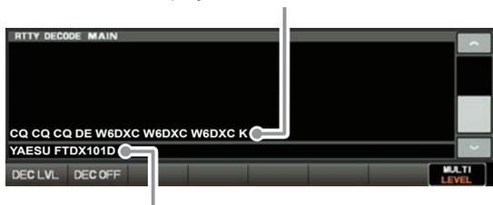
Displays text entered into the RTTY sending memory.
