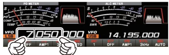
Touch “MHz” or “kHz” area of the frequency display to confirm. If there is no operation within 3 seconds, the frequency will be fixed.
