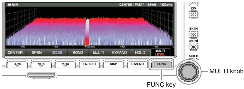
Press the [FUNC] key to call up the function screen for setting various functions. The setting menu (page 88) is also called from the function screen. Press again to return to the normal operation screen. Touch a MENU item, or rotate the [MULTI] control knob to make a selection.
