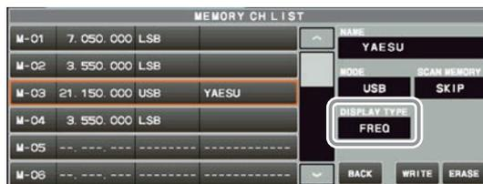
4. Rotate the [MULTI] knob to select the desired display type.
