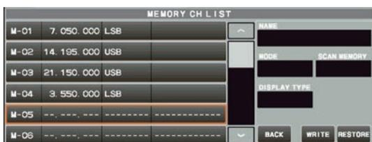
4. Press and hold the [V▶M] key to store the frequency and other data into the selected memory channel.
