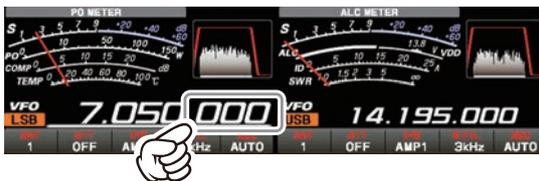
2. Enter the frequency using the numeric keys.
