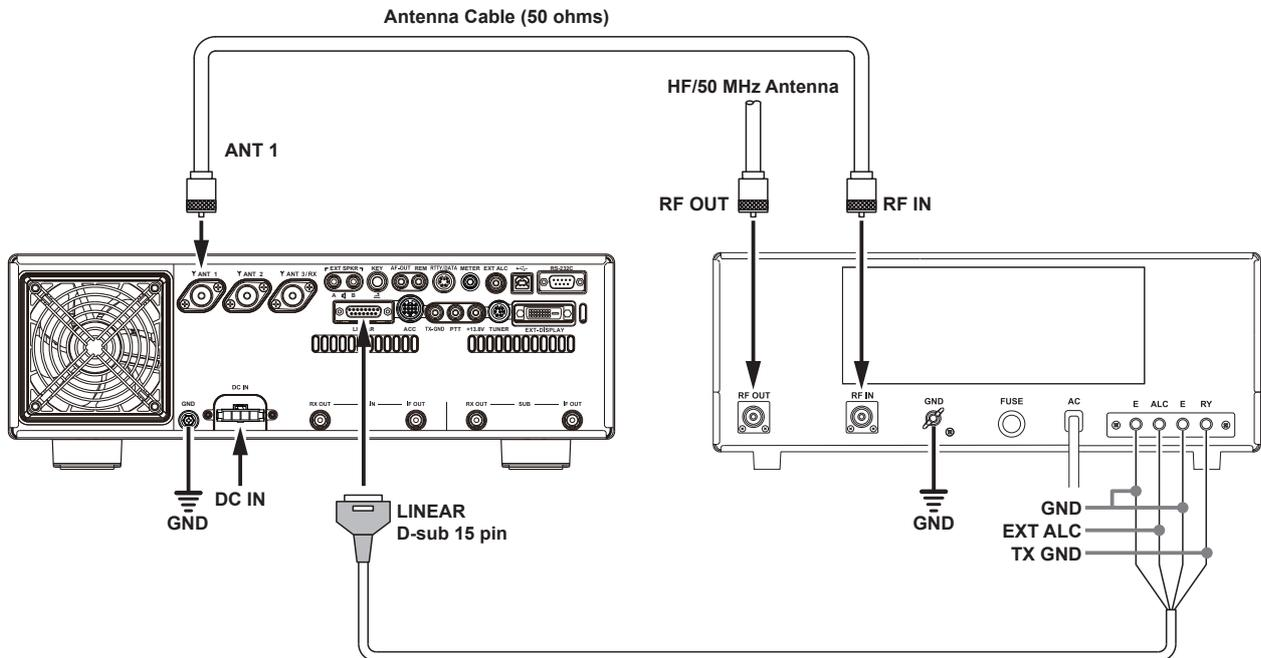
The figure above shows the FTDX101MP rear panel connections to other linear amplifiers.
