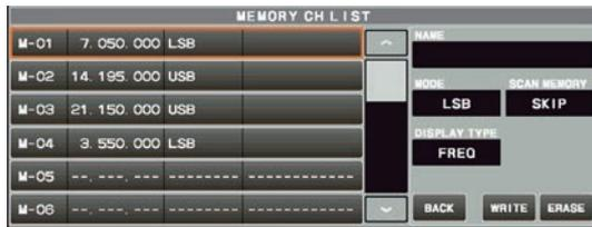
2. From the channel list, touch and select the memory channel and check, or change the operation mode.
