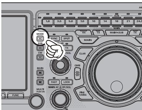
2. The operation MODE selection screen appears on the display, then touch [PRESET]. Touch [PRESET], the setting will be confirmed and then the operating screen will return.
