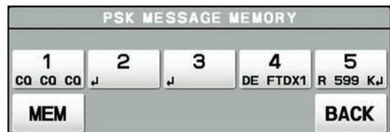
3. Touch [1] through [5] key, depending on which PSK Text Memory Register message you wish to transmit. The programmed message will be transmitted on the air.
