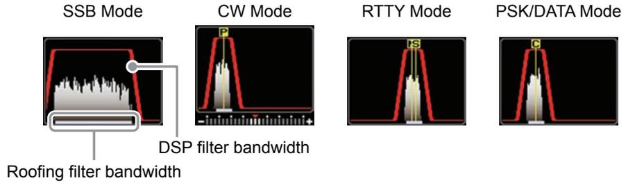
**i** Touch the filter function display to toggle between “normal display” and “magnified display”. Touch again to return to the “normal display”.
