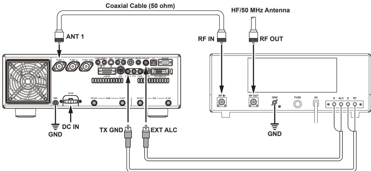
The figure above shows the FTDX101MP rear panel connections to other linear amplifiers.
