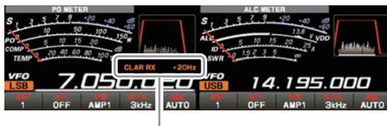
When the receive frequency is offset by +20 Hz.
