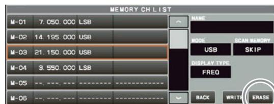
4. Press the [V▶M] key to erase the contents of the selected memory channel.
