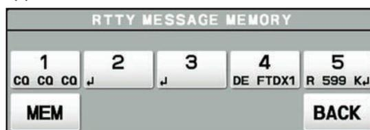
3. Touch [1] through [5] key, depending on which RTTY Text Memory Register message is to be transmitted. The programmed message will be transmitted on the air.
