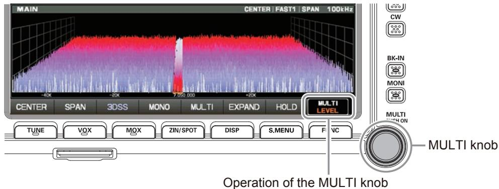
The following settings and operations can be performed with the [MULTI] control.
