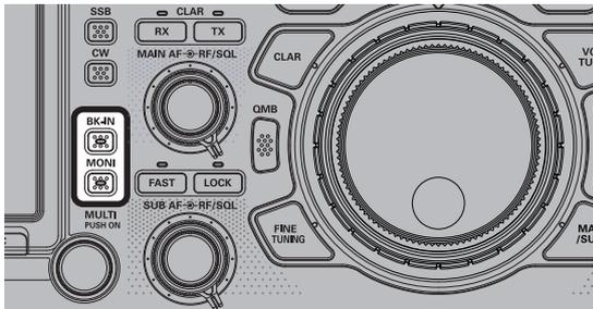
3. Rotate the Main Tuning Dial knob to select the desired operating frequency.
